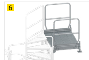
Optional assembly of another descent platform
