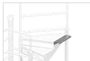
Alternative options for mounting a descent step
