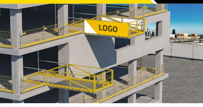
Unloading platform TUP - it is used to increase safety and facilitate transport of building materials to building tiers. It consists of componentry that is bolted together. Its mobility is significantly facilitated by easy assembly and disassembly which also reduces transport costs.
